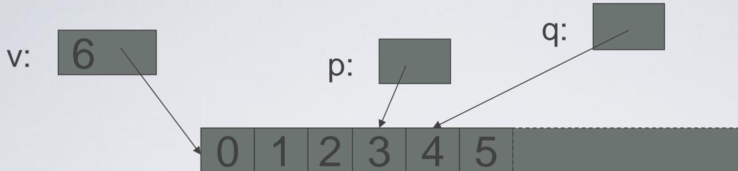
***p=v.insert(p,99);***      *// leaves p pointing at the inserted element*
