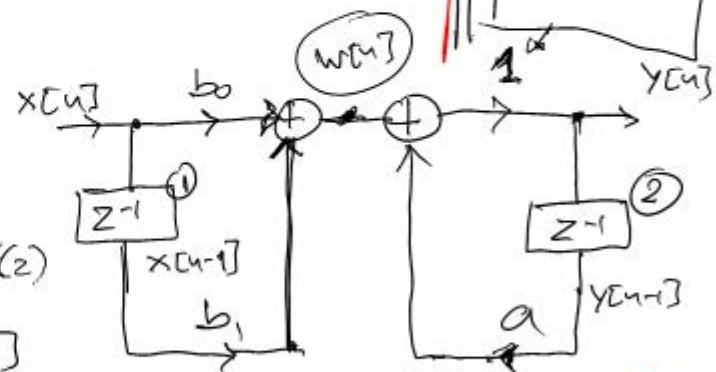
$$H(z) = \frac{b_0 + b_1 z^{-1} + b_2 z^{-2} + \dots + b_M z^{-M}}{1 - a_1 z^{-1} - a_2 z^{-2} - \dots - a_N z^{-N}}$$
