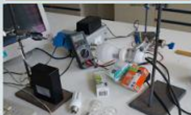
Figure 1. Apparatus used to make comparative calculations of temperature, electric current and spectral radiance
