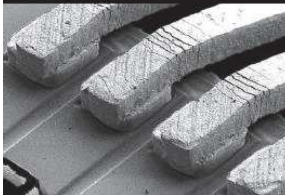
Integrated circuit bond pads ---2.5kV--- 500X ---SEI Mode
