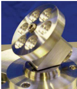
Rotary device to ensure uniform coating
