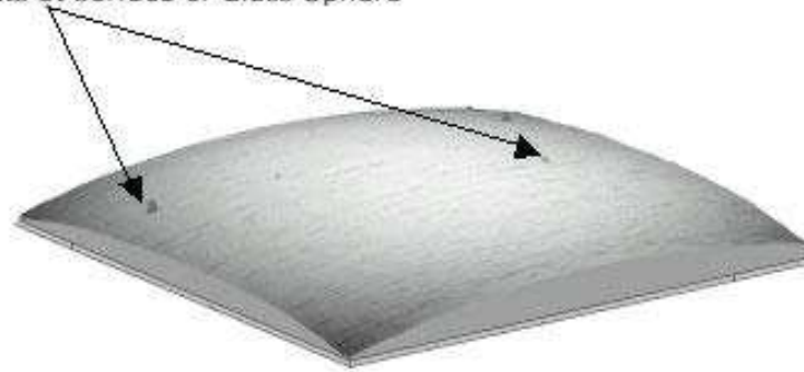
Defects at surface of Glass Sphere
