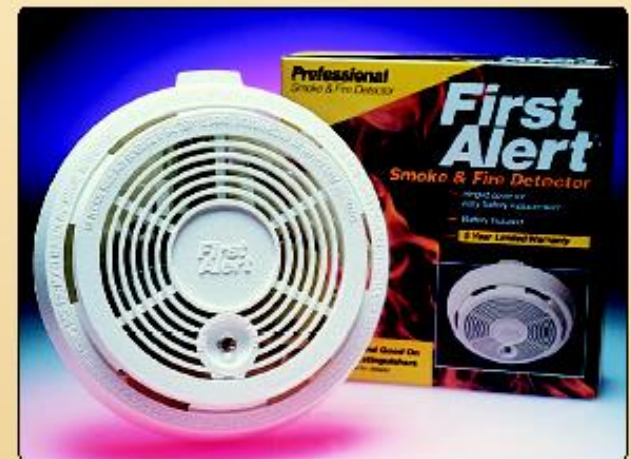
A household smoke detector uses radioactive americium-241. This alpha emitter has a half-life of 470 years. In a smoke detector the emission ionizes smoke particles to activate the alarm. (Charles D. Winters)
